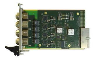
The TCP886 is equipped with a transparent PCI/PCI-X to PCIe Bridge which is capable of performing data transfer with a bus width of up to 64 bit at bus frequencies of up to 133 MHz depending on the product order option and the system backplane configuration.
