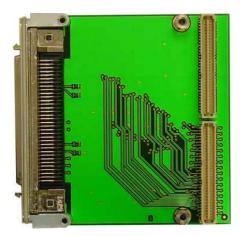
The TPIM003 distributes all 64 PMC back I/O lines to a 68 pin SCSI-3 type connector located in the EMI front panel. Additional GND pins are inserted by solder jumpers at pin 9, 26, 43 and 60 of the 68 pin SCSI-3 type connector. The routing and I/O signal mapping of the TPIM003 is optimized for differential pair routing.
