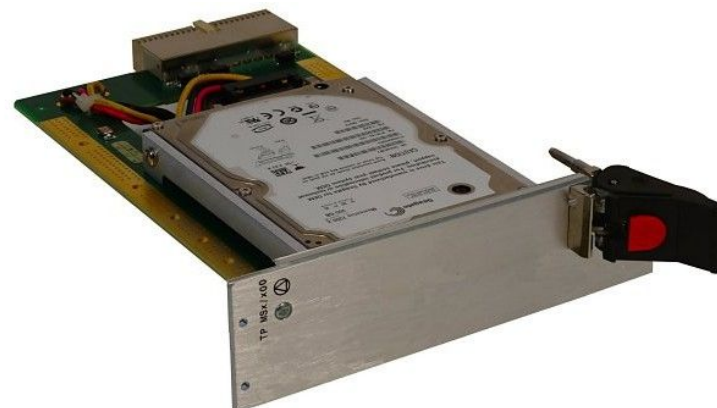
3U 8HP Expansion board with two SATA300 drives (fits into a slot to the right of the controller board)
