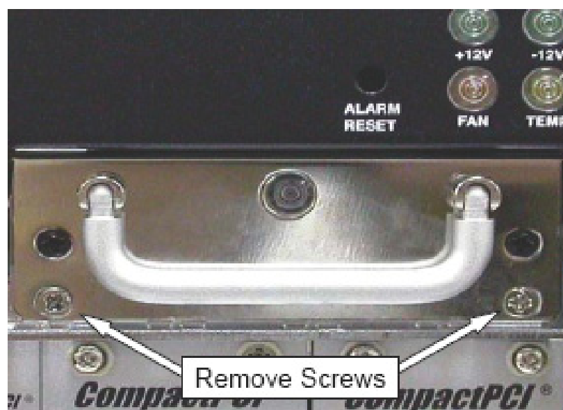
Figure 4-5: Remove the screws securing the fan module
