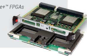
Based on the latest AMD 20nm FPGA family, the **IC-FEP-VPX6e** enhances the Front-End Processing (FEP) Interface Concept product line.
